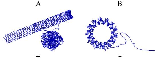
Figure 6: The role of embodiment. (A) Wheel size 1.1 (default 1.0). After a very irregular initial phase, the robot enters an aligned wiggly pattern, running at first to the right and then back toward the left lower corner. (B) Wheel size 1.125 leads to a circular pattern again. Parameter:  $\varepsilon = .001$ ,  $\alpha = 3$ .
