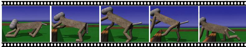
**Video 10.4: DOG “playing” with barrier.** The DOG video demonstrates the playful manner of exploring the world in the homeokinetic learning scenario. Note that the robot has nothing but its joint angle sensors as source of information about its body and the environment. The DOG is protected by an invisible box on its back preventing it from falling over. The video can be watched at <http://playfulmachines.com>.
