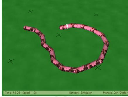
motor. A motor value of zero corresponds to a straight configuration and  $-1$  and  $1$  are associated with the fully deflected positions at  $\pm 90^\circ$  off center. The robot is underactuated, meaning the power of the motors is not sufficient to move the joints independently of each other to any position. This effect is especially strong at the joints in the middle of the robot. In order to change the joint angle, both halves of the body have to be moved.
