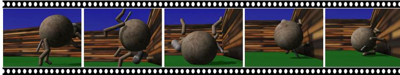
**Video 10.6: The HIPPODOG — The effect of the anatomy.** The HIPPODOG with its spherical trunk is developing more active and jumpy motion patterns due to its specific anatomy. The video can be watched at <http://playfulmachines.com>.
