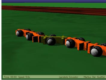
**Video 3.3: Emerging cooperativity in a chain of TWOWHEELERS.** The arena has no obstacles. Control is completely decentralized, but the individual wheels spontaneously cooperate in the working regime close to the effective bifurcation point. The video can be watched at <http://playfulmachines.com>.
