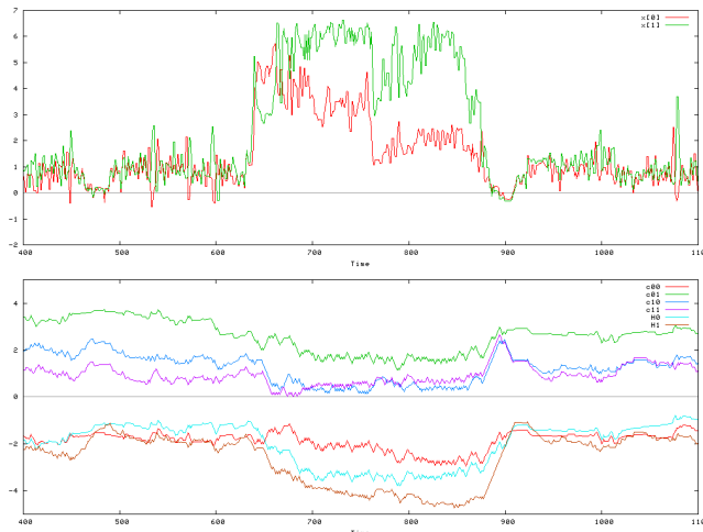
Fig. 3. Environment sensitive behaviour. Top: Sensor values from left and right infrared sensor over time; Bottom: Parameter values over time; Until time 640 we observed rocking (oscillatory) motion with a short break at time 480. Then the robot was set into a corner. The infrared sensors measure much shorter distances since they see the walls. At time 870 the robot was pulled back into free space. After each change of the environment the robot was calm for a while (low sensor fluctuation) and probed the new environment, however after a short time the robot rocked again.
